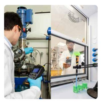
**MultiLine® IDS portable meters** are robust and waterproof according IP 67. Depending on the model they have one or two USB interfaces and color dis-
